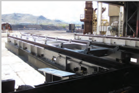
Here's a Ducking-Dog Style Charge Table. Billets are supplied by mobile equipment.
