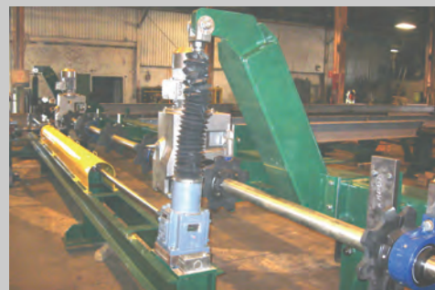
About one-third of the Charge Table pivots down to place a plate onto a roller table.
