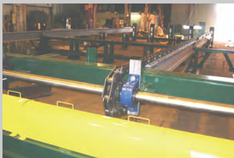
This is the drive end of a Plate Charge Table. Rugged steel mill chain transports plates.
