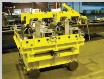
This Transfer Car is part of a Press Feed System.
