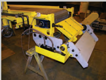
A Sorting Conveyor which rotates and pivots to distribute product to several different bins.
