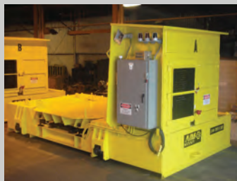
The diesel-electric generator is enclosed in a "doghouse".
