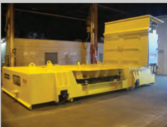
One of two Scrap Bucket Transfer Cars—both with weighing.
