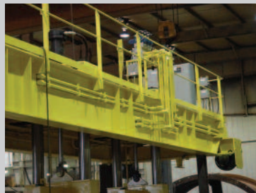
Bridge Beam and Hydraulic Piping
