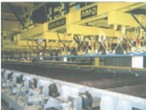
Plate Being Lifted off of AIM's Roll Conveyor
