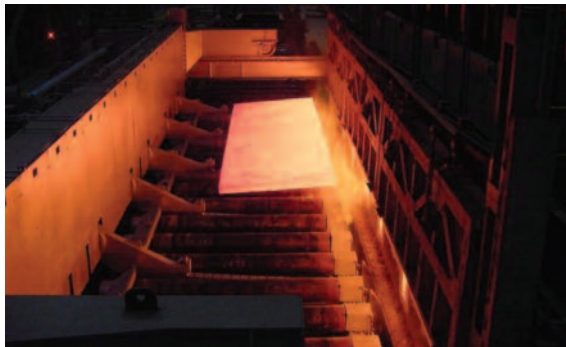
Furnace Extractor Handling a Hot Slab
