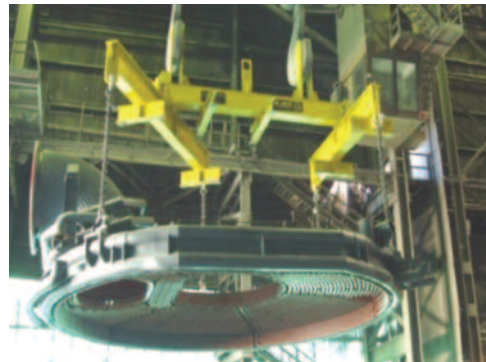
Lifting Rig for an Electric Furnace Roof
